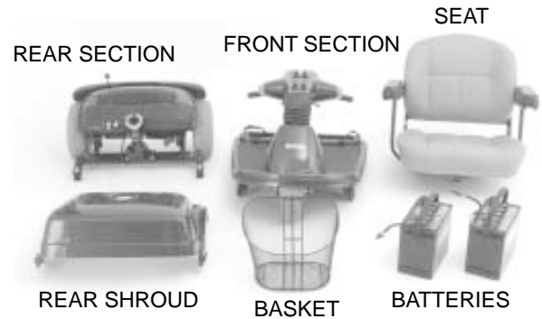
Figure 15. The Maxima Disassembled
