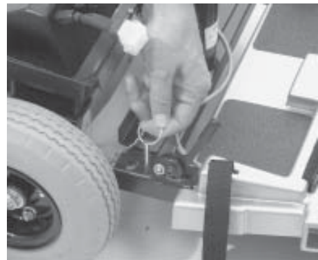
FIGURE 22. REMOVE BALL DETENT PINS WITH RINGS
