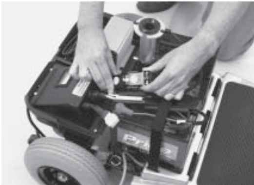
FIGURE 18. DISCONNECTING THE MOTOR HARNESS
