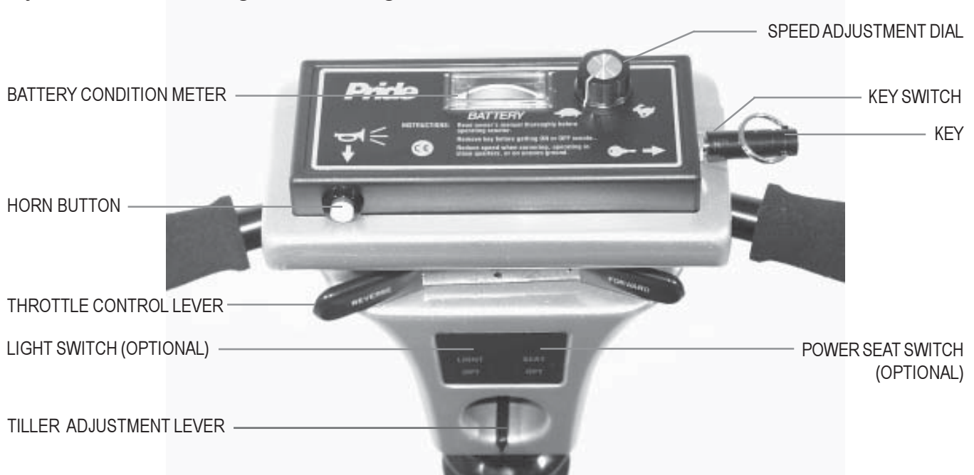
FIGURE 6. CONTROL CONSOLE ASSEMBLY
