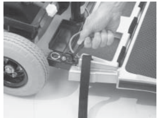
FIGURE 21. PUSH LOCKING LEVERS FORWARD
