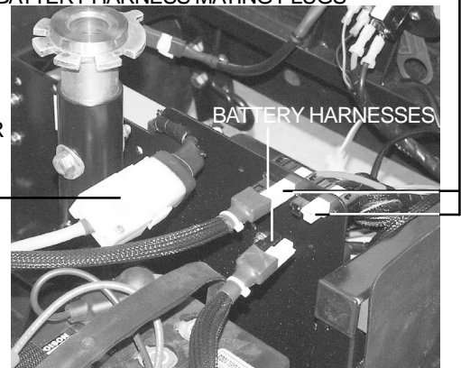
Figure 12A. Disconnect Battery Harnesses
