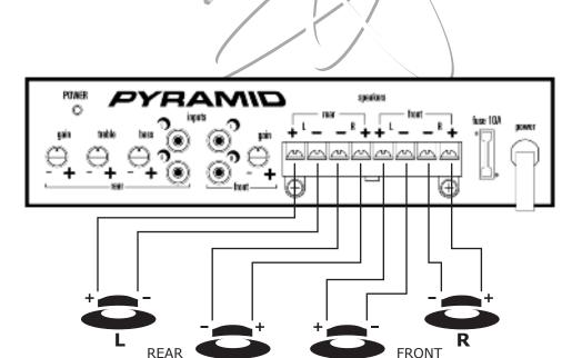
NOTE: The PB442X is not capable of having bridged outputs. Bridging the outputs will damage your amplifier!
