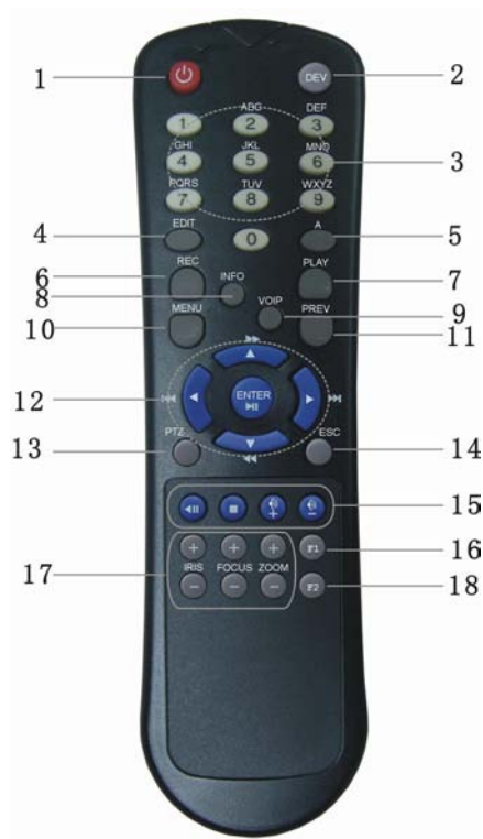
Fig 3-2 IR Remote Control Layout
