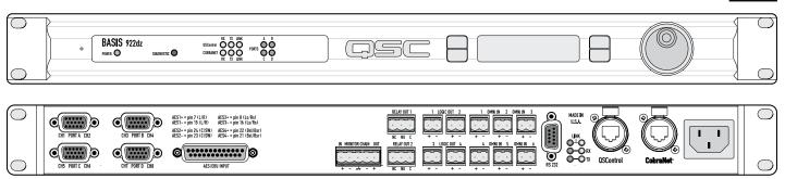
QSControl.net, QSC's next generation network audio system, achieves the seamless integration of the company's signal transport, control, processing, and monitoring technologies. QSControl.net brings together QSC's digital, power amplification and loudspeaker products into a unified system that enables the user to administrate it all via a fully integrated graphical user interface. The new generation BASIS devices are designed to operate under the company's QSControl.net platform.
