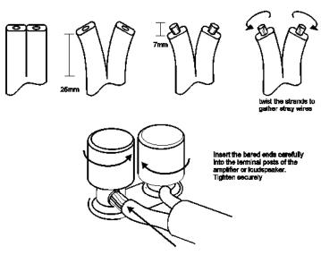
When estimating the length of loudspeaker cable, provide sufficient to enable access and tidy securing. Some cables are quite heavy and should be placed so that they do not cause undue strain on the binding posts of the subwoofer.
