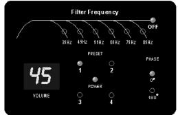
**Volume:** Press the Volume + key to increase the volume level. Press the Volume - key to decrease the volume level of the subwoofer. The volume range on the front panel display varies from 00 (minimum) to 99 (maximum).
