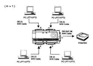
Fig. A 4-IN- 1 -OUT configuration
