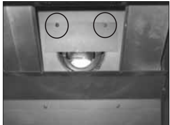
Figure 8.5 With the baffle removed, remove the two screws located in the back of the firebox. Reuse the screws to install the flue restrictor.
