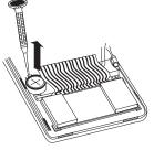
Position the new battery so the positive (+) side is up, then insert it into the battery compartment.
