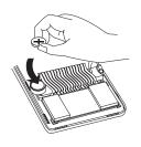
Snap the front and back case halves back together, then replace the screws.
