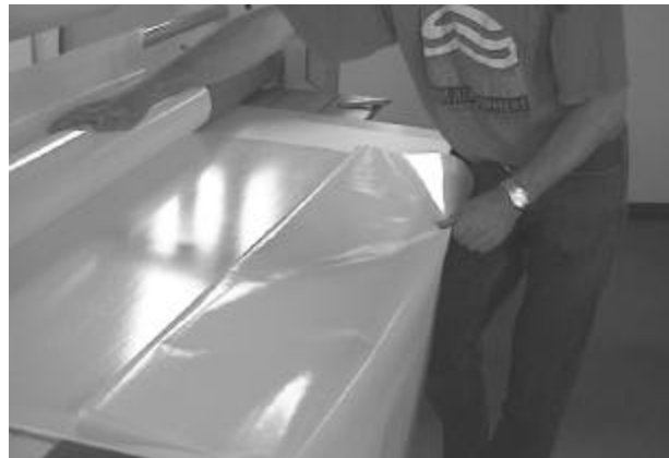
Figure 13. Removing the release liner from a Decal
