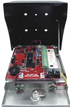
Unique faceplate hinge allows for easy installation.
