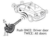
**NOTE:** If a door is not opened within 30 seconds of unlocking, all doors will relock for safety.
