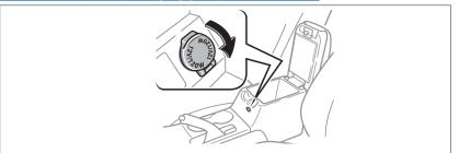
Designed for car accessories. Key must be in the "ACC" or "ON" position to use.
