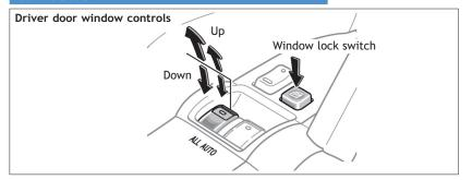
**Automatic operation (all windows)** Push the switch completely down or pull it completely up and release to fully open or close. To stop window midway, lightly push the switch in the opposite direction.
