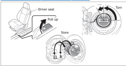
NOTE: Tighten cap until one click is heard. If the cap is not tightened enough, Check Engine " (CHECK " indicator may illuminate.
