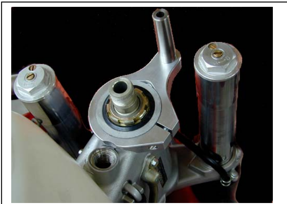
Frame bracket must be flush with top of head tube
