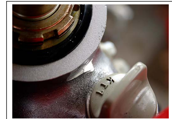
File the casting flaws both front and rear until smooth, round and allowing the bracket to sit down flush
