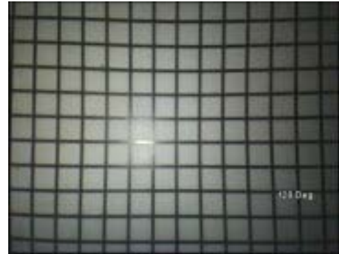
120° optical tip, distortion correction on
