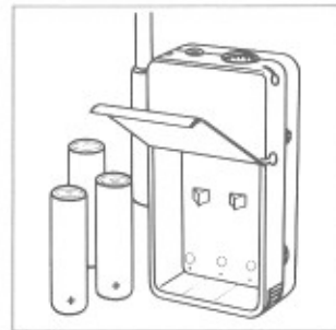
Fig. 2: Inserting the Batteries
