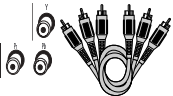
Component video jacks and cables are often color-coded (red, blue, and green).
