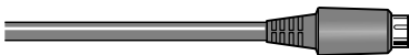
If your TV has an S-Video jack, connect the S-Video cable (supplied). S-Video provides better video quality than composite video (the yellow jack).
