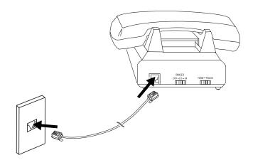
**Note:** The USOC number of the jack to be installed is RJ11C.
