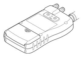
Warning: Set ALKALINE/RECHARGEABLE to RECHARGEABLE for use only with nickel cadmium (Ni-Cd) or nickel metal hydride (Ni-MH) rechargeable batteries. Never attempt to recharge nonrechargeable batteries. Non-rechargeable batteries can get hot or explode if you try to recharge them.
