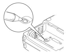
Install 2 AA batteries, matching the polarity symbols (+ -).
