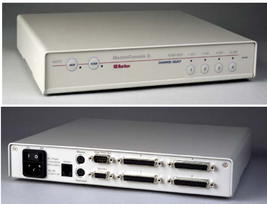
Figure 1 MCC4 – Front and Rear Views
