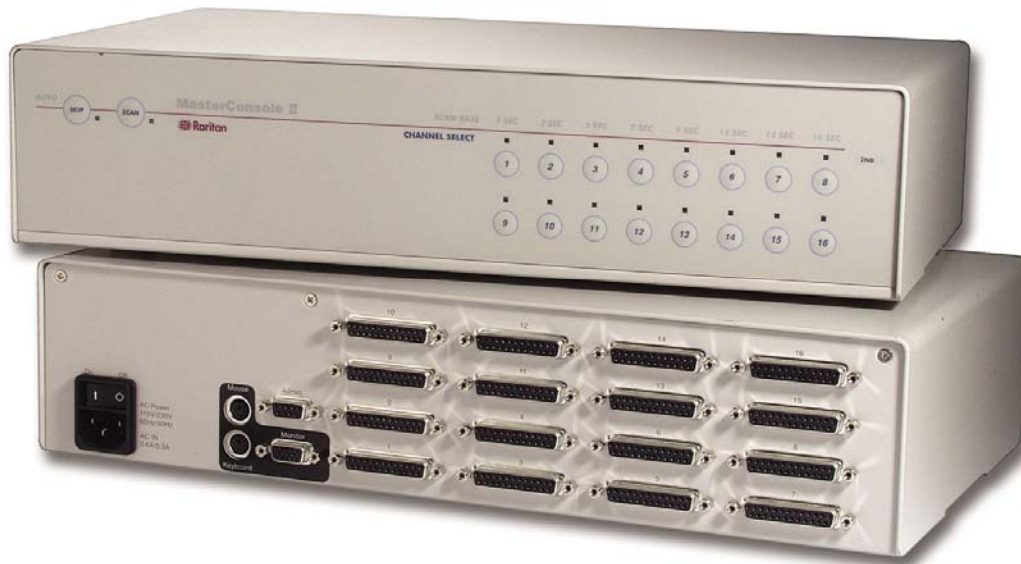
Figure 3 MCC16 – Front and Rear Views
