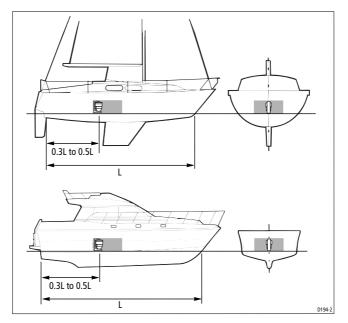
The compass is normally bulkhead mounted below decks. However, it can be mounted above deck on steel vessels. Although it is weatherproof, performance may be impaired due to the increased motion if it is mounted above deck.
