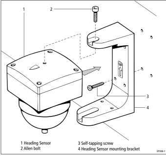
6. Pass the Allen bolt (2) through the aperture in the top of the Heading Sensor mounting bracket (4) and tighten using the Allen key supplied.
