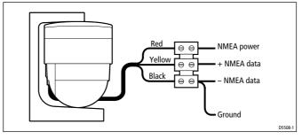
Check the handbook supplied with NMEA 0183 compatible equipment, to determine the correct pin connections for the heading sensor input. For example, the connections for a XX Radar are shown in the following diagram.
