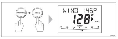
In Wind Vane mode, the SmartPilot will then adjust the boat's heading to maintain the locked wind angle.
