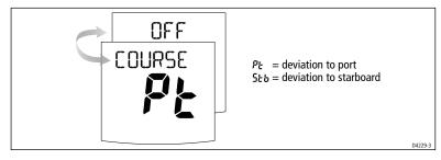
The SmartPilot warns you when you have been off course from the locked heading for longer than 20 seconds. It shows whether the deviation is to port or starboard.
