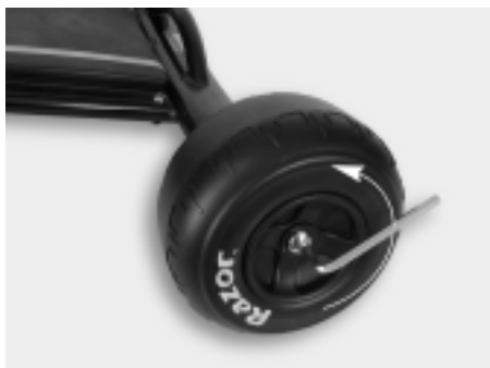
Figure 3e. Tightening the backwards threaded axle.
