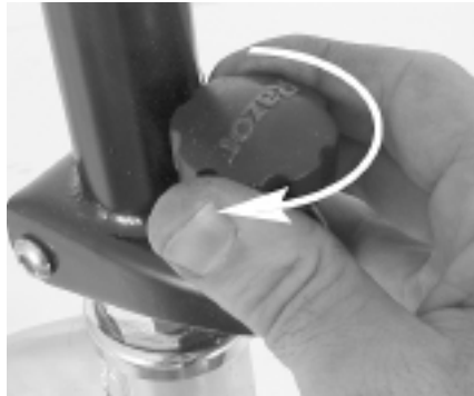
Figure 4. Tighten the locking knob.
