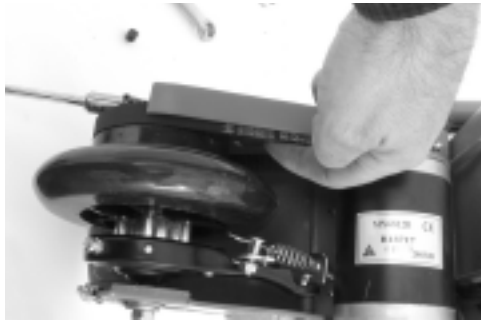
Figure 31. Tighten both axle adjusters the same number of turns to tension the drive belt and to approximately maintain the centering of the wheel.
