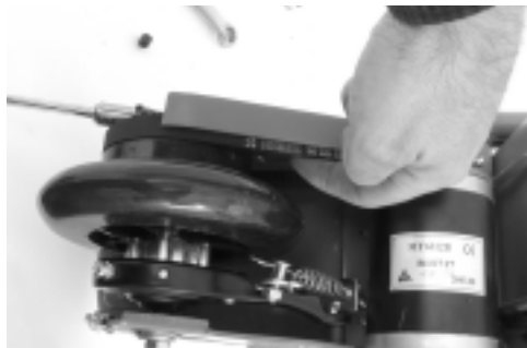
Fig 13 and 14. Tighten both axle adjusters equally, 1/8 to 1/4 turn until the belt or chain is properly tensioned.
