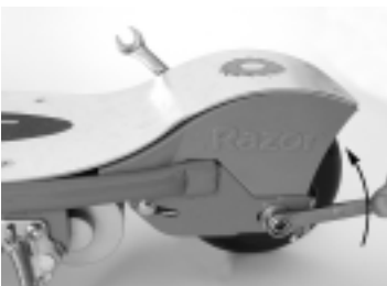
Fig. 19 & 20. Loosen the axle and push the wheel forward in the slots to loosen the belt as shown.
