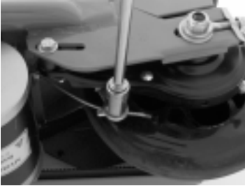
Fig. 15. Loosen brake cable anchor and disconnect the cable.
