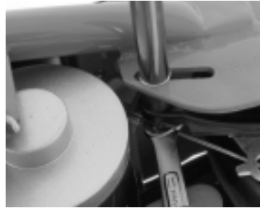
Fig. 16. Loosen brake housing anchor and disconnect.
