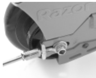
Fig. 18. Loosen both axle adjusters an equal amount, about five turns.
