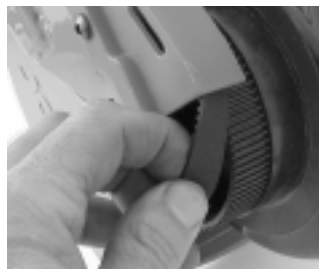
Fig. 19 & 20. Loosen the axle and push the wheel forward in the slots to loosen the belt as shown.
