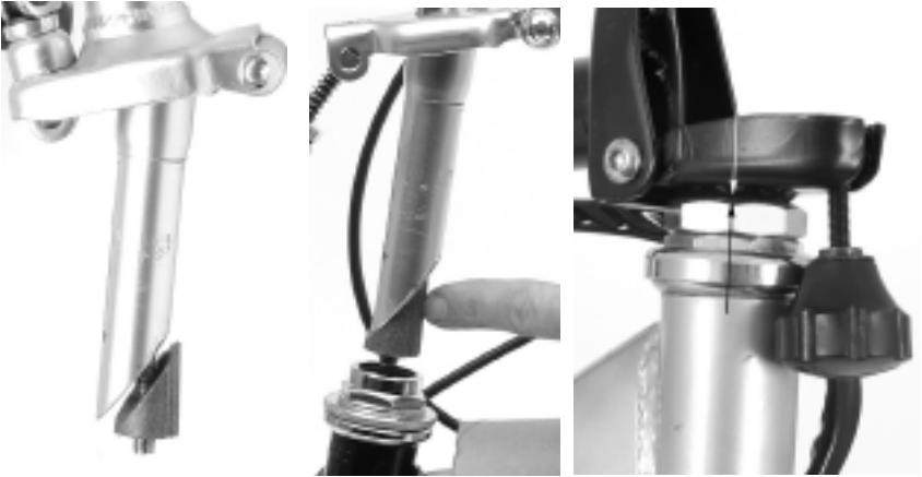
Figure 2a, 2b and 2c. Inserting the handlebar quill into the fork.
