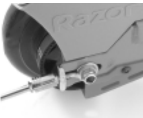
Fig 13 and 14. Tighten both axle adjusters equally, 1/8 to 1/4 turn until the belt or chain is properly tensioned.
