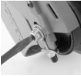
Figures 29 and 30. Install the axle adjusters and axle nuts. Tighten until they just barely hold the hardware in place.
