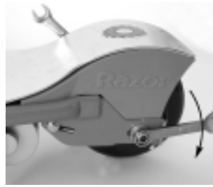
Figures 29 and 30. Install the axle adjusters and axle nuts. Tighten until they just barely hold the hardware in place.
