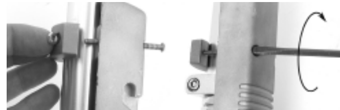
Installing the screws and tightening the clamps.
