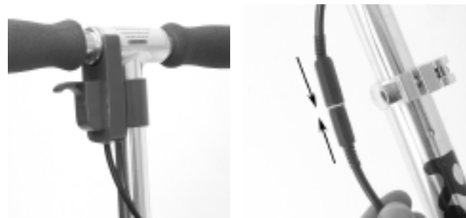
Final connection of the wiring (right)
