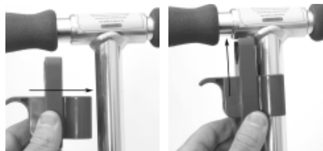
Attaching the power control
