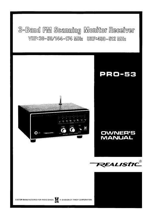
Your PATROLMAN PRO-53 scanning receiver is a completely solidstate VHF/UHF superheterodyne receiver using dual-conversion. It is capable of automatically scanning eight crystal controlled channels. Some special features are: crystal filter, ceramic filter, channel lockout circuit, skipper circuit, scan delay circuit and AC operation.
