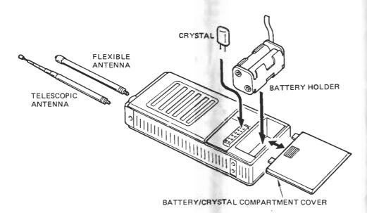
Two antennas are provided with the PRO-22: a flexible "rubber duck" antenna and a telescoping one. The flexible antenna is for use in cramped areas or wherever a longer antenna would get in the way. The telescoping antenna is for obtaining the very best possible reception from your receiver. The telescoping antenna must be extended fully for proper operation.
