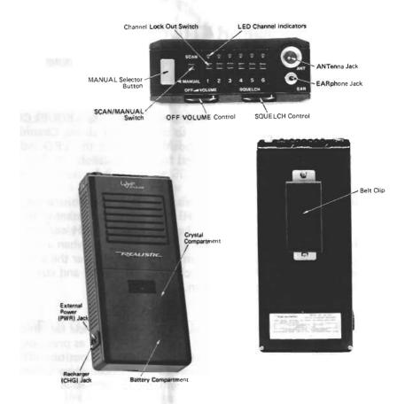
Battery Compartment holds the internal power source (4 type AA batteries).
