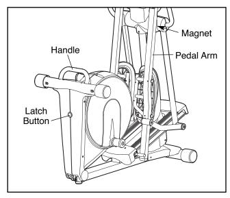
To use the elliptical exerciser, first hold the handle, press the latch button, and then lower the frame.
