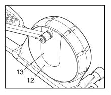
Cover (13) using a flat screwdriver. Next, remove the four screws (not shown) from the center of the left Disc (12). Gently rotate the Disc Cover and the Disc away from the elliptical exerciser.
