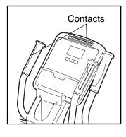
rate, hold the handgrip pulse sensor with your palms resting against the metal contacts. **Avoid moving your hands or gripping the contacts tightly.**
