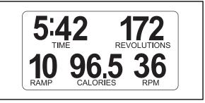
The upper right corner of the display will show the distance you have pedaled, in total revolutions. The display will also show your heart rate when you use the handgrip pulse sensor (see step 5 on page 15).
