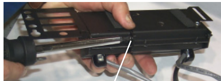
Secure the 2 boxes together with one screw.
