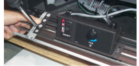
Secure left side with 2 screws.
