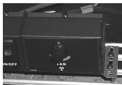
Secure right side with 2 screws.
