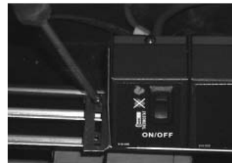
Secure left side with 2 screws.
