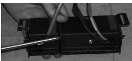
Secure the 2 boxes together with one screw.
