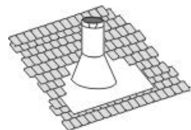
Diagram 11: The upper half of the flashing is installed under the roofing material and not nailed down until the chimney is installed. This allows for small adjustments.
