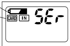
The LCD monitor displays the message "Waiting to communicate."
