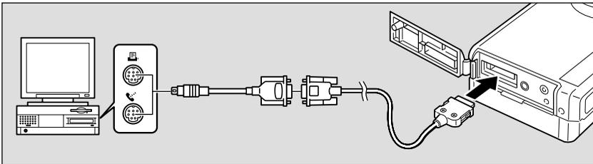
The above diagrams illustrate typical connections to the Ricoh digital camera RDC-5000.
