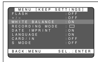
The settings of the items for which Keep Setting is programmed will be retained even when the camera is turned off.
