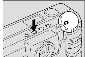
The flash mode setting is displayed on the LCD monitor or on the LCD panel. When you press the shutter release button, the subject is shot in slow synchro mode with the flash activated. The flash LED lights (red) as you press the shutter release button lightly.
