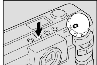
The flash mode setting is displayed on the LCD monitor or on the LCD panel. Press the shutter release button to record the image without firing the flash.
