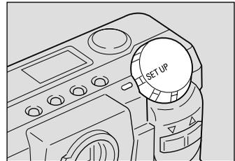
**2 Press the or button to select [FORMAT] and press the ENTER button.**
