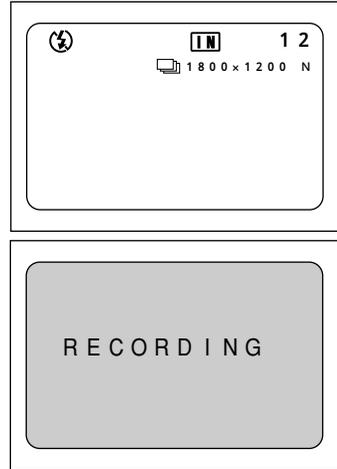
When you continue pressing the shutter release button, the camera will take one picture about every second continuously. Continuous shooting stops when you release the shutter release button, and the images that have been shot so far are recorded automatically. The message “RECORDING” appears on the LCD.
