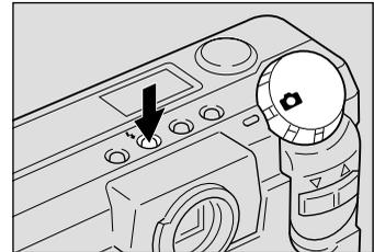
The flash mode setting is displayed on the LCD monitor or on the LCD panel. Press the shutter release button to take the picture using the flash. The flash LED will light (red) when you press the shutter release button lightly.
