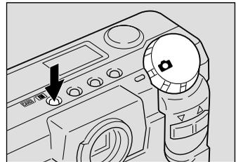
The recording destination changes each time the **CARD/IN** button is pressed. Press the **CARD/IN** button and make your choice.
