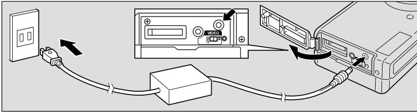
❶ Check that the camera is turned off, and then open the terminal cover.
