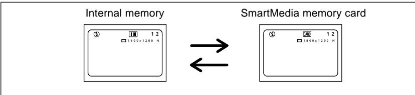
\* When the SmartMedia memory card is inserted, the **CARD** will be displayed.
