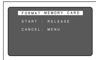
**Note** • A SmartMedia memory card with a write protect pad attached to it cannot be formatted. Remove the pad to format the SmartMedia memory card.
