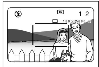
**Note** When the digital zoom function is enabled, shots taken will be recorded in 640 × 480 pixel format.
