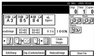
❖ When the 1000-sheet finisher is installed
