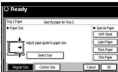
**2 Enter the vertical size of the paper using the number keys, and then press the [#] key.**
