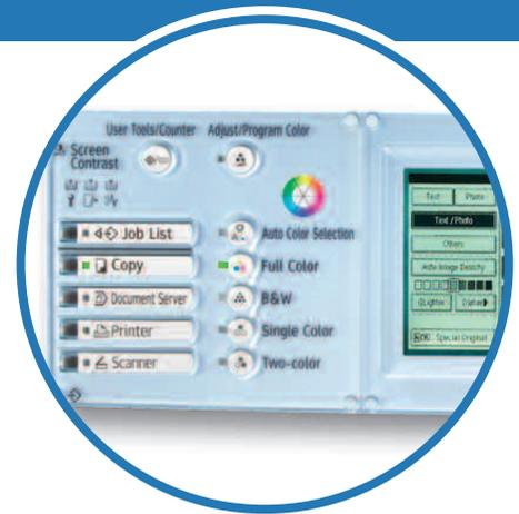
The Ricoh Aficio Color 5560V control panel features an intuitive design with clearly labeled hard keys and easy-to-understand icons. This same ease of use is available through the Ricoh RPCS (Refined Print Command Stream) print driver.
