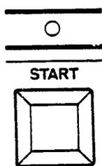
A light-touch pushbutton is used for smooth start/stop operation. Tempo Pilot Lamp illuminates at the first beat of every bar for indication of rhythm speed.
