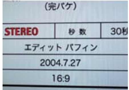
Photo 3. Image output from an ordinary HD VTR via HD-SDI and down-converted by the VC-300HD. Parameters and other settings were not adjusted.
