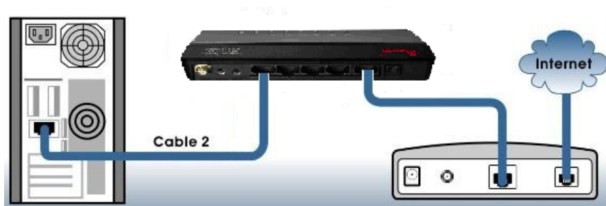
RNX-N400LX, PC, and Modem Rear View (WAN Port and LAN port Connection diagram between PC, Wireless Router and Modem)
