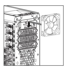
NOTE: If you use only one 5.25" bay, you can install one 120mm fan onto three 5.25" steel cover with screws.
