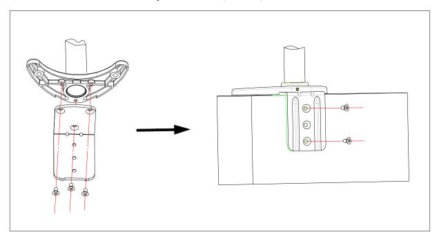
Step 2 –Insert the mount arm[02] to base[01] WARNING:TIGHTENING TORQUE[01-d] BEFORE INSERT THE MOUNT
