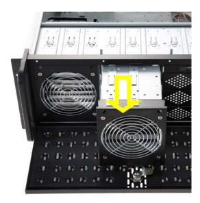
**2.** Pull the middle module out from the front panel
