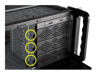
Using a flathead screw driver to press the Yellow circle to move the front panel out.
