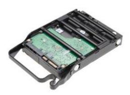
**4.** The HDD tray can be easily clipped onto 3.5" HDD.
