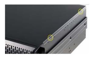
Remove the screws from each side of the Chassis. (two on each side)
