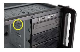
**5.** You can slide the ODD back in to complete the installation.
