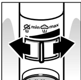
Set the variable steam control to required steam volume. Steam can only be produced when the thermostat is in the red cotton/linen zone. Allow iron to heat up (light goes out) before activating the variable steam control. Reduce or set variable steam to min. when ironing at low temperatures to avoid water leakage or spitting.
