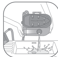
Rinsing out the boiler D
