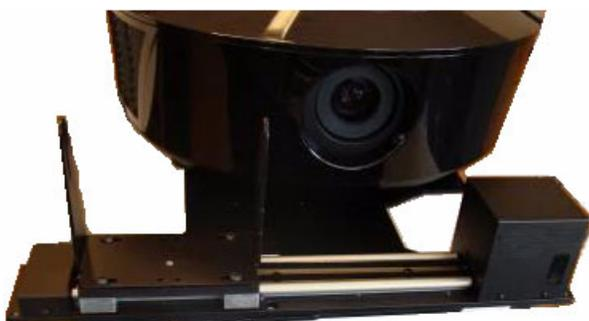
**Attaching the Security Hooks:** To help stabilize and support the added weight of the Anamorphic Lens and Lens Transport Assembly, the attachment plate includes two security hooks and related hardware for attaching the front part of the plate to the ceiling above.
