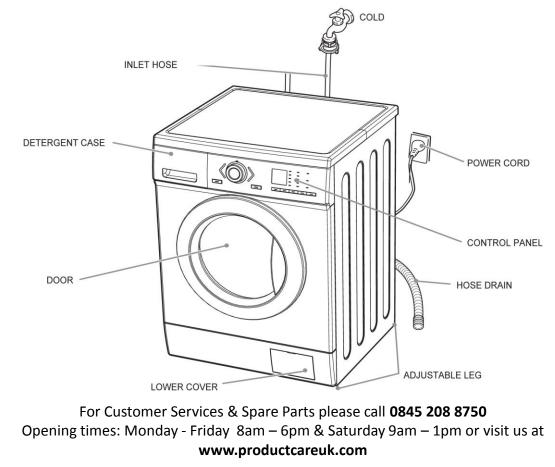
1. Before operating the washing machine, remove the 3 transportation screws and rubber spacers. If the screws are not removed, it may cause heavy vibration, noise and product malfunction, (voiding the guarantee).
