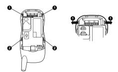
■ Release the front panel by moving the retention lugs (2) if necessary and pushing them with a pen for example.
