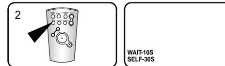
3. To start the delayed recording, press the START/STOP button.
