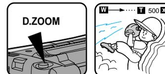
**Note:** The D.ZOOM ON/OFF function will not operate in EASY, REC or CUSTOM mode.
