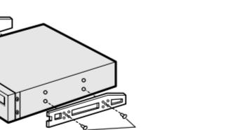
**2 Remove the plate from a free expansion slot and install the CD-ROM drive, as shown in the illustration.**
