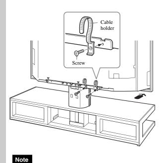
The two cable holders and two screws are supplied with the TV.
