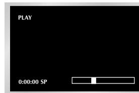
Press the INFO. button to see the current status of the VCR deck, as well as the tape counter position and record speed.
